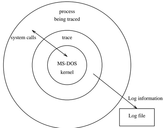
Figure 3: Structure of the system running *trace*.
