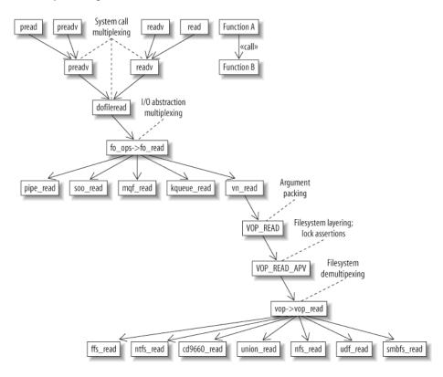
Figure 2: Layers of indirection in the FreeBSD implementation of the read system call
